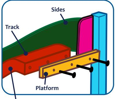
Lateral flange at 90 ° to the track for bolted installation to panels.
